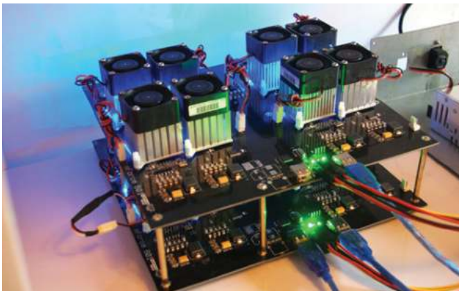
Figure 14.2: FPGA used for cracking hashes
