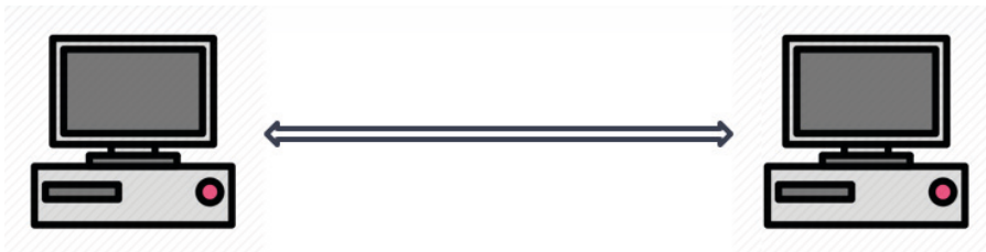
Figure 3.1 – The simplest form of a network – two interconnected computers
