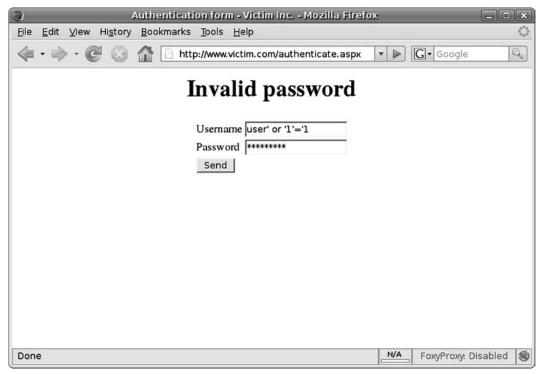
Figure 2.8 shows a flaw in the authentication system of Victim Inc. The application shows different error messages when it receives a valid username, and moreover, the username field seems vulnerable to SQL injection.
